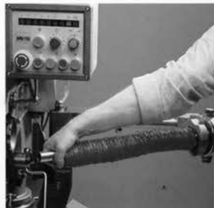
The swing-out filling horn allows for easy casing change.
